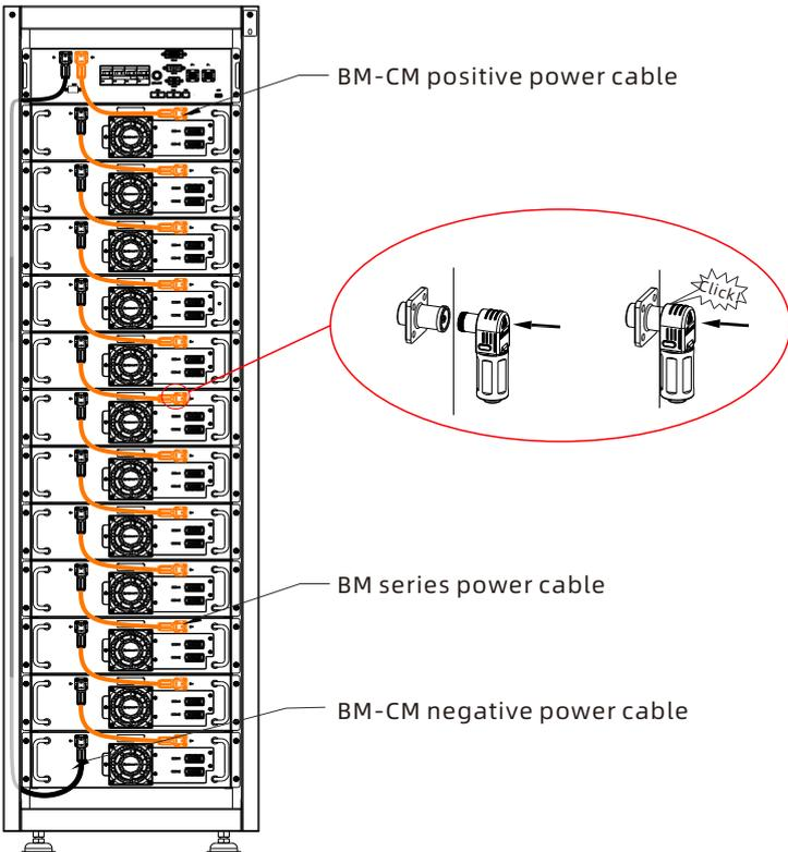
Please measure the voltage of each battery pack accurately before connecting the power cable. The bottom battery pack "B-" terminal is connected to the high-voltage box "B-" terminal. The "B +" terminal of the top battery pack is connected to the "B +" terminal of the high-voltage box.
