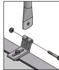
Depending on the panel width, the clamps B1 and B2 must be positioned inwards or outwards. The correct orientation for each panel width is shown on the next page.
