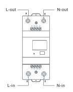
The Ingress Protection rate is IP51, So meter must be installed in door. The whole installation chart shows as below:
