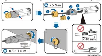
Figure 5-36 Installing anti-theft components for the Smart Dongle
