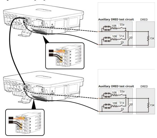
Figure 7-4 Wiring diagram for the DRM function
