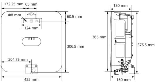
Figure 4-1 Mounting bracket dimensions
