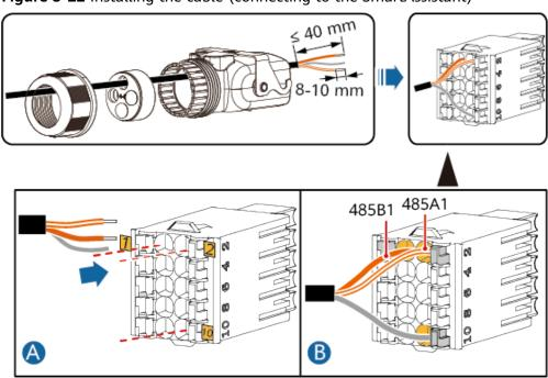
Figure 5-22 Installing the cable (connecting to the SmartAssistant)
