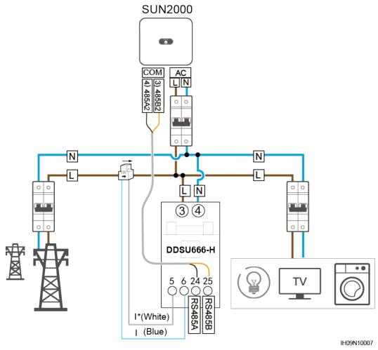
Figure 5-29 Connecting cables to the DDSU666-H power meter
