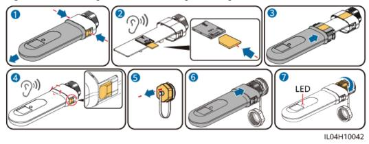
Figure 5-38 Installing anti-theft components for the Smart Dongle
