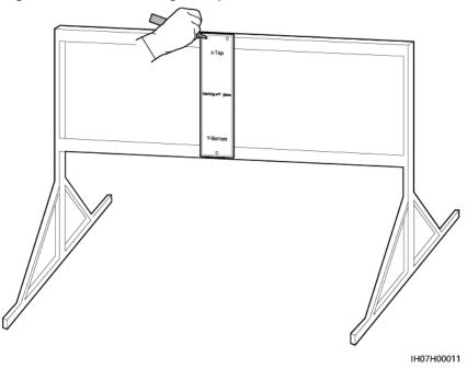
Figure 4-11 Determining hole positions
