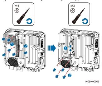
Figure 8-2 Removing the faulty fan(Type 2)
