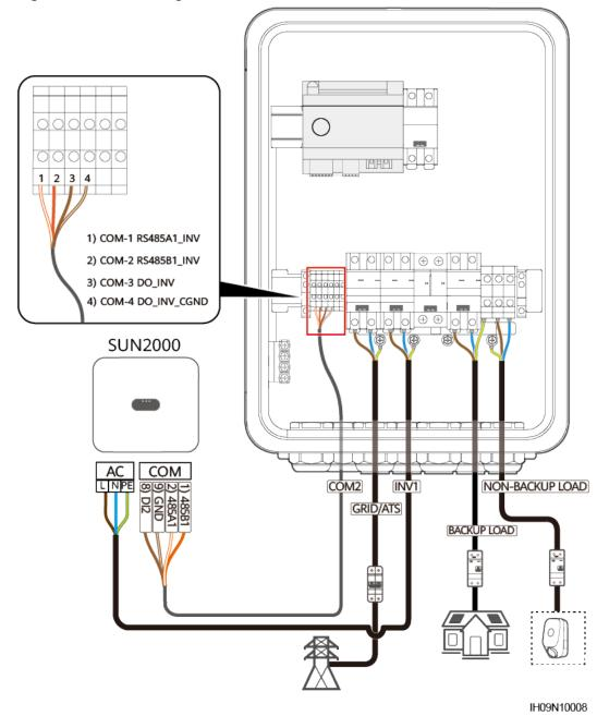
Figure 5-25 Connecting cables to the SmartGuard
