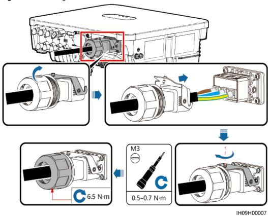
Figure 5-5 Securing the AC connector
