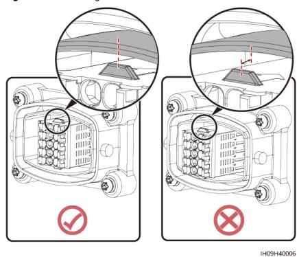
Figure 5-18 Installing the connector block
