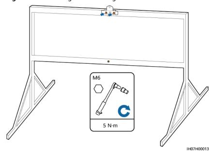
Figure 4-13 Securing the mounting bracket
