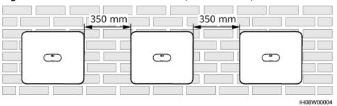
Figure 4-4 Triangle installation mode (recommended)
