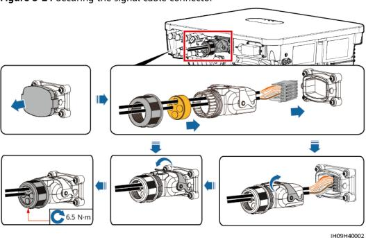
Figure 5-24 Securing the signal cable connector
