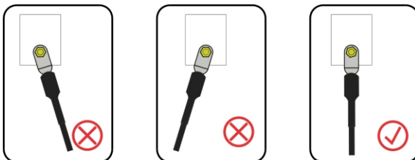
Figure 5-5 Ensuring the cables are parallel
