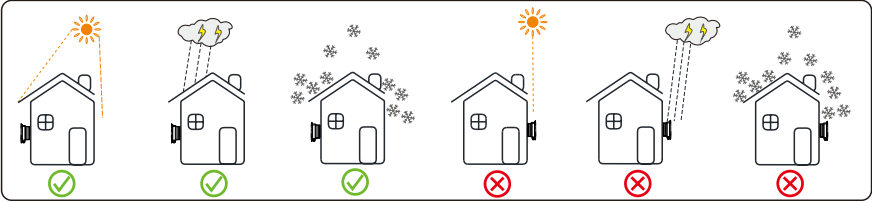
Figure 4-2 Installing an awning and clearance requirements
