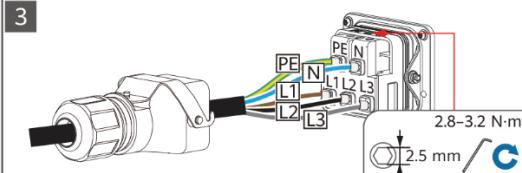
**EN-GB** Secure the power plug with a screwdriver. Apply paint or take other protection measures.
