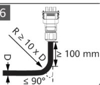
**EN** Connecting an AC Output Power Cable
