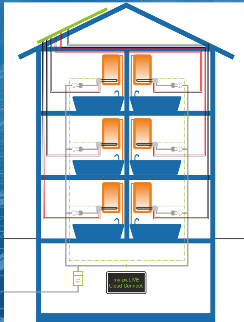
Autonomous hot water with ELWA
