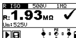
Figure 5.7: Example of an insulating resistance measurement
