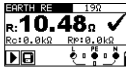
Figure 5.35: Example of an earthing resistance measurement
