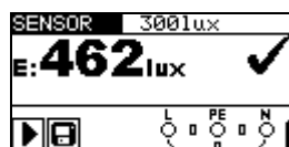
Figure 5.47: Example of a luminous intensity measurement
