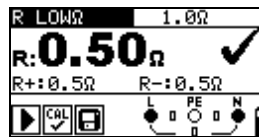
Figure 5.10: Example of a low-impedance measurement RLOWΩ
