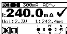
Figure 5.20: Example of a tripping current measurement
