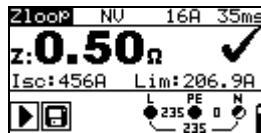
Figure 5.25: Example of a loop impedance measurement
